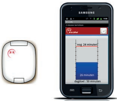
Figure 1 The It's LiFe! tool: accelerometer and app on a smartphone 7
